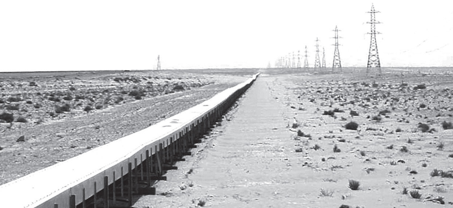
Western Sahara has the world's longest conveyor belt: From the large Bou Craa phosphate mines, phosphates are transported a distance of more than 100 km, ending up in the El Aaiún harbour, Western Sahara's capital. Source: http://www.bersek-productions.no
